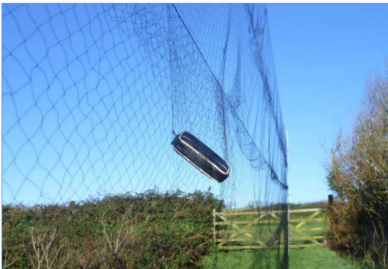
Figure 10. The depth of a shelf pocket on a Merlin, 18m, 70 denier, 2-ply nylon, mist net.
